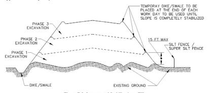
Figure B.2: Incremental Stabilization - Fill
