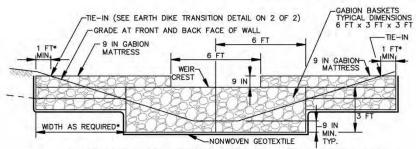
\*ONE BASKET OR MULTIPLE MATTRESSES NEED TO EXTEND FROM THE GABION/EARTH INTERSECTION (TIE IN) TO A MINIMUM 1 FOOT BEYOND THE TIE IN.
