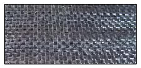
**Woven Slit Film Geotextile**
