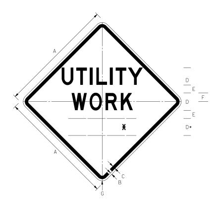
\* REFER TO DISTANCE DETAILS IN WORK AREA SECTION FOR LINE 3 MESSAGE AND DIMENSIONS
