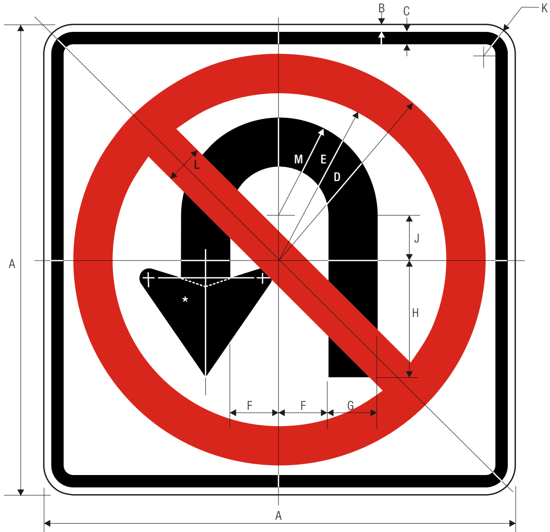
R3-4 U-TURN PROHIBITED
