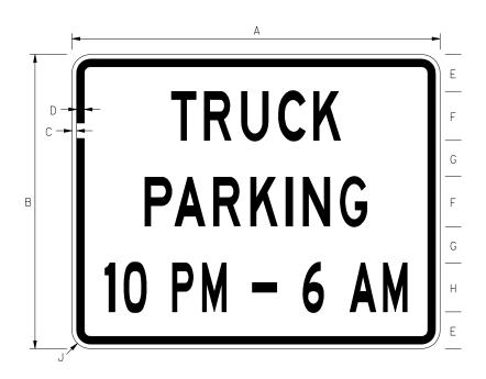
NOTE: SIGN ONLY TO BE INSTALLED BELOW D4-2 AND SHALL MATCH WIDTH OF D4-2.
